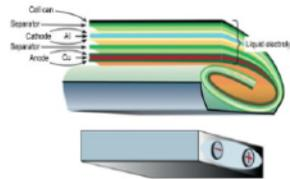
A prismatic design indicate a flat battery design. The stacks can be wound (as shown in the photo) or stacked (with alternating cathode/separator/anode structure). The stacks are usually inserted into rigid casing to form prismatic containers
