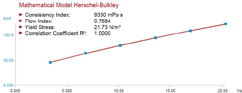
Calculated Herschel-Bulkley parameters to determine the flow behavior of slurry
