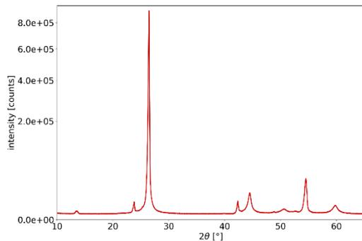
Diffractogram of a graphite anode material
