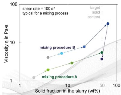
Comparison of mixing procedures A and B in terms of total solid fraction and viscosity, at constant shear rate
