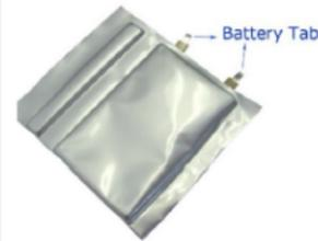
Rather than rigid metallic casing, conductive foil-tabs are welded to the electrodes and seal the battery fully. The stacks inside can be wound or stacked. Swelling and gassing could be a concern for pouch cells.
