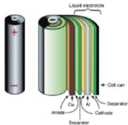
A spirally wound design (jelly-roll). Designated by size, e.g. 18650 cylindrical battery (Diameter: 18.6 mm, length: 65.2 mm; code for cylindrical shape: 0)
