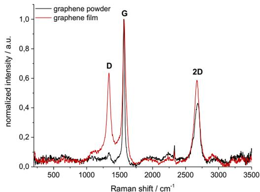
Raman spectra of graphene powder (black) and a graphene film (red).
