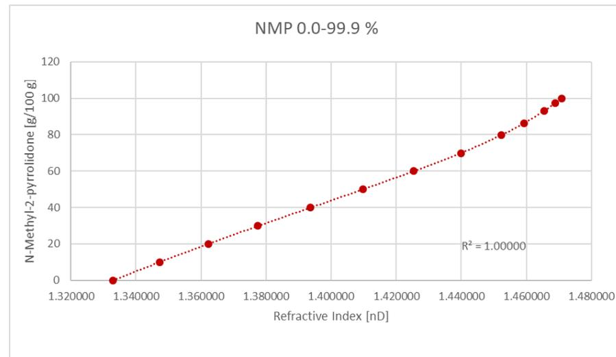
Refractive Index of different NMP concentrations measured at 20 °C and 589 nm
