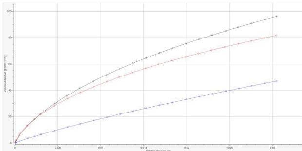
**CO<sub>2</sub> isotherm on 3 types of hierarchical carbon samples (micropores)**
