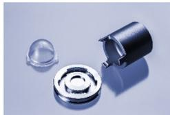
Sample holders for air-sensitive battery materials
