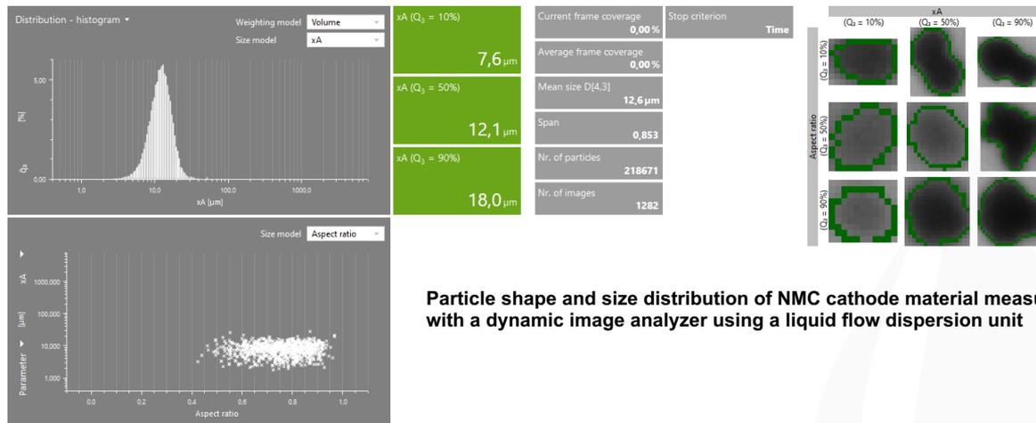
**Particle shape and size distribution of NMC cathode material measured with a dynamic image analyzer using a liquid flow dispersion unit**
