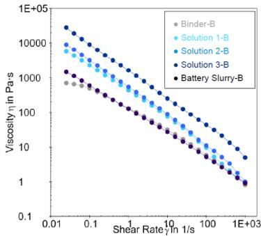
Viscosity curves measured after stepwise addition of components, representing the processing steps for mixing procedures A and B
