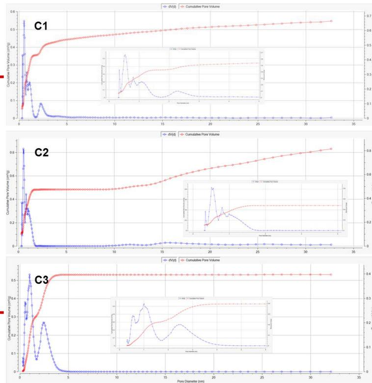
**Merged CO<sub>2</sub> (273 K) and N<sub>2</sub> (77 K) DFT pore size distributions (blue) and cumulative pore volumes (red) for three carbons**
