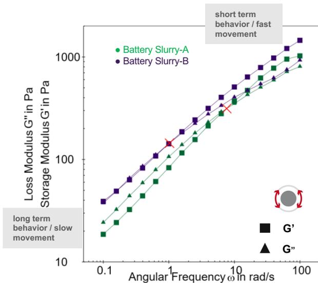
Frequency sweeps of sample battery slurry A and battery slurry B.
