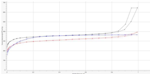
**N<sub>2</sub> isotherm on 3 types of hierarchical carbon samples (mesopores)**
