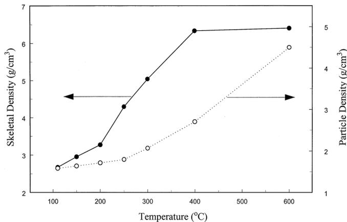
Increase of skeletal density with increasing thermal treatment of nickel oxide electrode material
