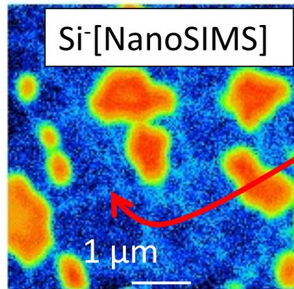
NanoSIMS is capable of detecting Si along with grain boundary in ceramics, contrary to SEM-EDX, EPMA
