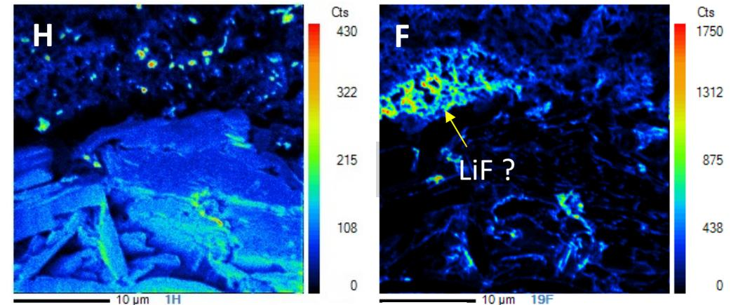
Evaluation of Li, which is hard to detect by EDX, is enabled by NanoSIMS
